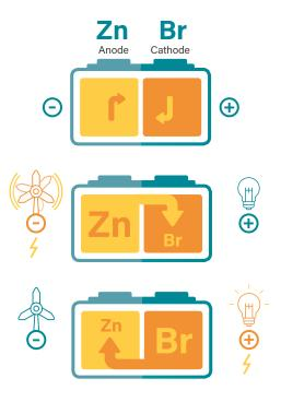
The zinc-bromine flow battery is a hybrid flow battery fuelled by the reaction between zinc and bromide.
